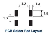
Package is Thermoplastic. Dimensions are millimeters.
